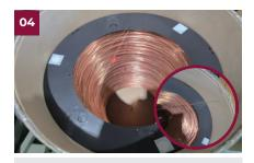
Cut the fixed wire at the starting section.
