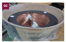
Arrange the sealed plastic film so that it wraps around the outside of the drum.
