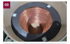
Remove the press plate, silica gel, and fixing spring. (As there is no inner drum, all auxiliary materials must be removed from the pack and used externally.)\*
