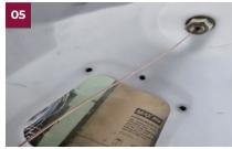
Insert the wire into the cap nipple and push it forward to the feed roller.
